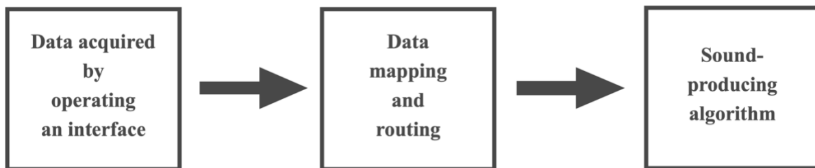
Figure 1. The structure of data-driven instruments.
