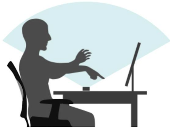
Figure 10. Leap Motion hand-tracking interaction zones (Reallusion 2024).
