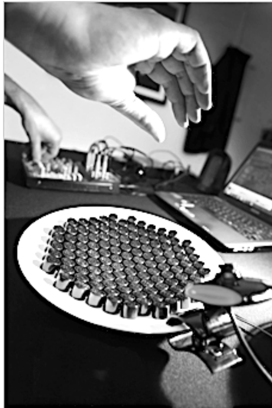
Figure 2. Syntact™ front-end - concavely shaped transducer array
