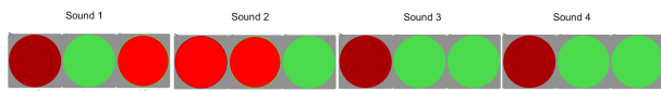
Figure 2. The display in this Max patch indicates that the recorded buffer is playing from sound component 1, after the performer left sensor 1, while sound component 2 is currently recording and playing, as sensor 2 is reacting to the performer's presence. Sensors 3 and 4 are inactive, neither playing nor recording.
